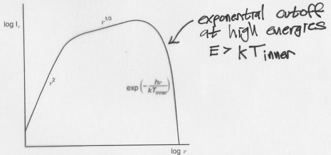
Figure 16.7. A schematic representation of the emission spectrum of an optically thick accretion disc. The exponential cut-off at high frequencies occurs at frequency  $\nu = kT_{\text{inner}}/h$ , where  $T_{\text{inner}}$  is the temperature of the innermost layers of the thin accretion disc.
