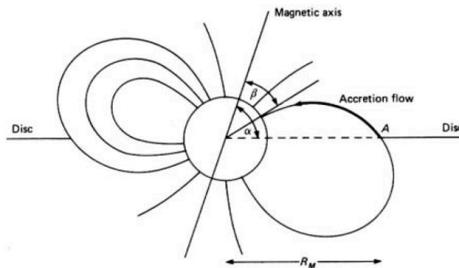
Figure 8: Accretion in a strong ( $\sim 10^{12}$  Gauss) magnetic field. Note that the accretion disc is held off the neutron star surface by the centrifugal barrier formed by the rotating magnetosphere.<sup>23</sup>
