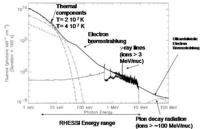
Figure 2: Theoretical HXR/GR spectrum
