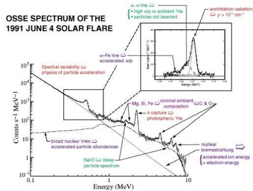
Figure 15: OSSE HXR/GR spectrum of the large 4 June 1991 flare summarising the different components seen in the 0.1 to 10 MeV range (from Share and Murphy 2000).
