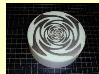
Fig. 7 Examples of ultra-wideband feeds. Left: the 300-3000 MHz feed for use on the 13.7 m telescope for the high frequency SRBS system. Right: a prototype sinuous feed under consideration for use on FASR antennas.
