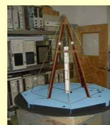
Fig. 7 Examples of ultra-wideband feeds. Left: the 300-3000 MHz feed for use on the 13.7 m telescope for the high frequency SRBS system. Right: a prototype sinuous feed under consideration for use on FASR antennas.
